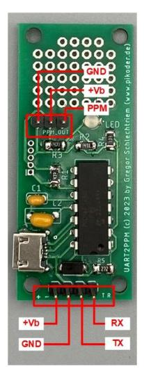
Please note: when powering the engineering board by USB, then +Vb would be about 5 Volts - 0.3 Volts (voltage drop diode). When powering the board via UART pins, the board would work with 3.3 Volts to 5 Volts.
